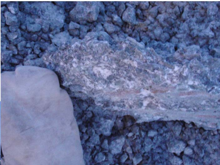
Photo 11 (mid left): Close up view of frozen 5/8” clear material being excavated in the North Dam key trench.
